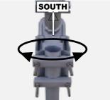
2.2 Align the dish to rotor's pole indicator.
