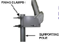
Fix the rotor to the supporting pole without tightening definitively the brackets.
