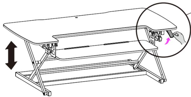
Based on the actual usage, press the handle grips simultaneously, and adjust the workstation to the proper height
