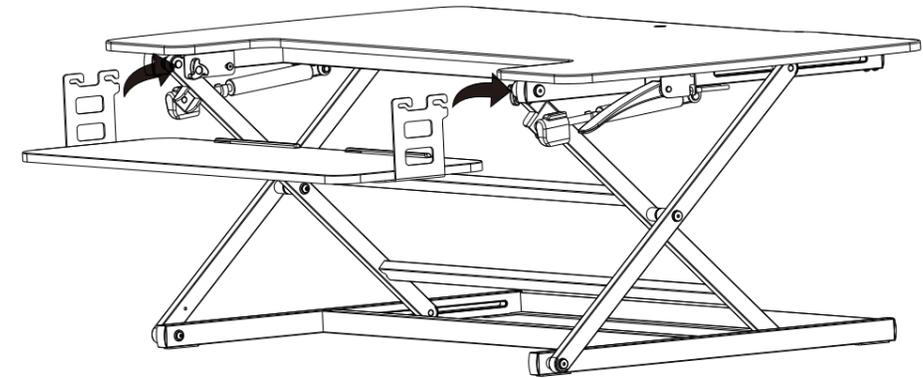
Hang the junction plate on the knob assembled and then tighten the knob
