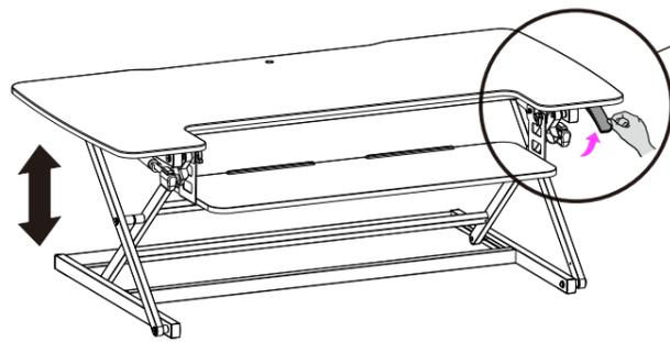
Based on the actual usage, press the handle grips simultaneously, and adjust the workstation to the proper height
