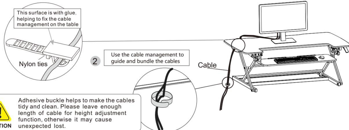
This surface is with glue, helping to fix the cable management on the table
