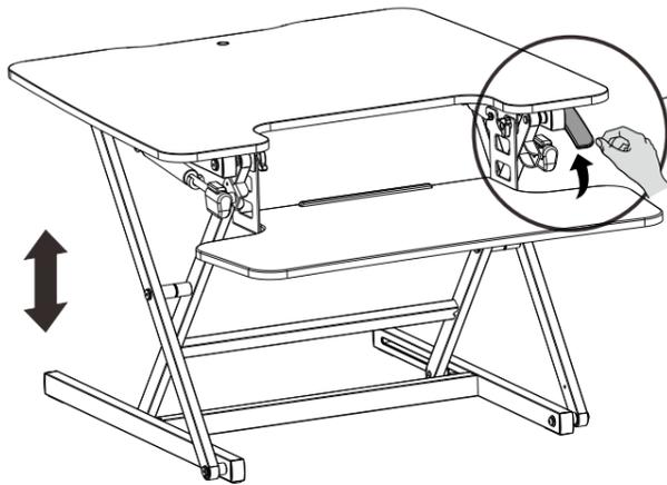
Based on the actual usage, press the handle on one side, and adjust the workstation to the proper height
