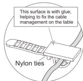
This surface is with glue, helping to fix the cable management on the table
