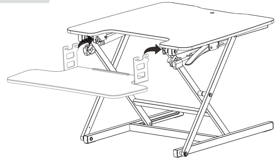
Hook the connection plate to the installed knob and tighten the knob.
