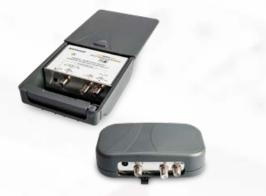
The **Stacker-Destacker** is the perfect solution to upgrade an old single-cable system with a twin (or quad) LNB to be used in combination with a dual input receiver (PVR) or 2 separate single input receivers. The advantage of using the Stacker-Destacker is that you don't need an additional cable. The Stacker converts the frequencies of the second input, so it is literally stacked above the frequencies of the first input. The Destacker converts the frequencies back to the original ones.
