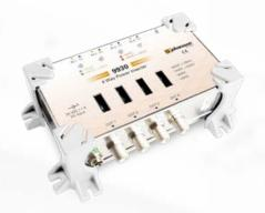
The 9930 is a **satellite power inserter**, which can be used to ensure a universal LNB is locked on the correct satellite band. Each of the 4 inputs can be configured to deliver the desired control signals (13/18V + 0/22 kHz). The selected control signal is indicated by a bi-color LED.
