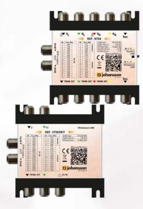
The 9734 has 4 satellite wideband input (for 1 quattro or 2 wideband LNB), passive terrestrial diplexer, 2 outputs with each 16 user bands.
