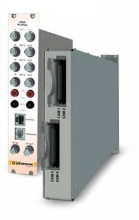
The new **satellite module** has 4 inputs allowing the reception of 4 different satellite bands per module. Because the module has 8 satellite tuners and a built-in multiswitch, reception of 8 different transponders coming from any of the 4 input satellite bands is possible.
