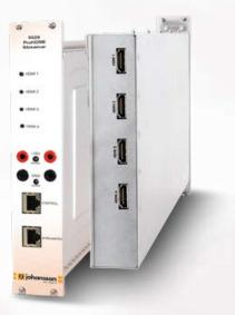
The 5520 is a **ProHDMI Streamer** with 4 HDMI inputs and 1 ethernet streaming port.
