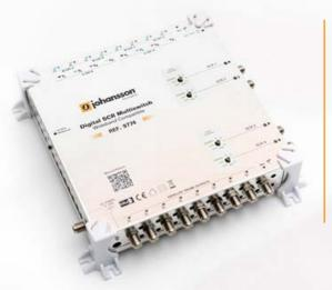
The 9775 has 8 satellite wideband inputs and 1 terrestrial input. This allows you to use 2 quattro LNBs or 4 wideband LNBs. The 6 SCR outputs have 10 user bands each. What makes the 9775 unique is the following: on each individual output, you can select the input and channel plan. This multiplies the available content and minimizes your equipment costs.
