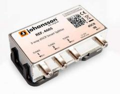
Standard **splitters** can give collisions when two commands come at the same time or when one of the set-top boxes uses a permanent high voltage. A smart splitter captures the commands of the different set-top boxes and serializes them to guarantee no collisions happen.
