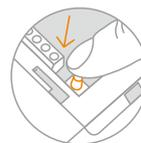
1. Press the enroll button of control panel, the control panel enters into enrolling status, the LED lights up in red. (Press again the enroll button within 20 seconds to exit enrolling state.)
