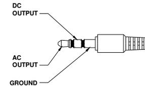
AC: Output voltage: 1Vrms corresponding to each range step.
