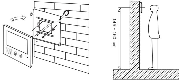
1. Using the screws to fix the mounting bracket on the wall.
